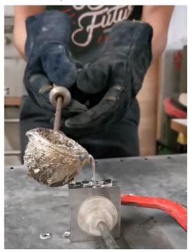
Casting was a simple case of pouring the hot metal into the mould. We got a fairly good finish from the castings when they were polished up. The buffing wheel was very aggressive when used with the pewter so some of the coins are a little bit out of round, need to be careful in the future! The internal parts of the Hackspace H came out much shallower than we wanted, next time we need to either make the shape bigger in the design or use a smaller tool when cutting the die to get extra detail.
