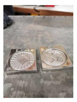
Once the CNC cuts on the mould were finished, we took it upstairs and used the Startrite Bandsaw to remove the excess clamping stock. Burrs were removed with the belt sander.
